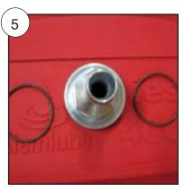
Insert Viton O rings (BS136) to grooves on both sides of coupling (400LP-C1)
