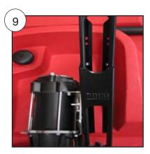
Attach nozzle holster to steel bracket on side of pump. Ensure that the holster is installed at a 65 to 75 degree angle so that the nozzle fits securely once attached to hose. Holster can be adjusted to suit manual or auto nozzles
